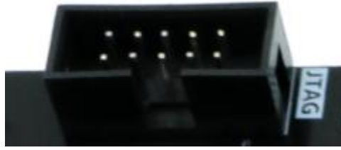
Figure 17-2: JTAG Interface on the FPGA board
