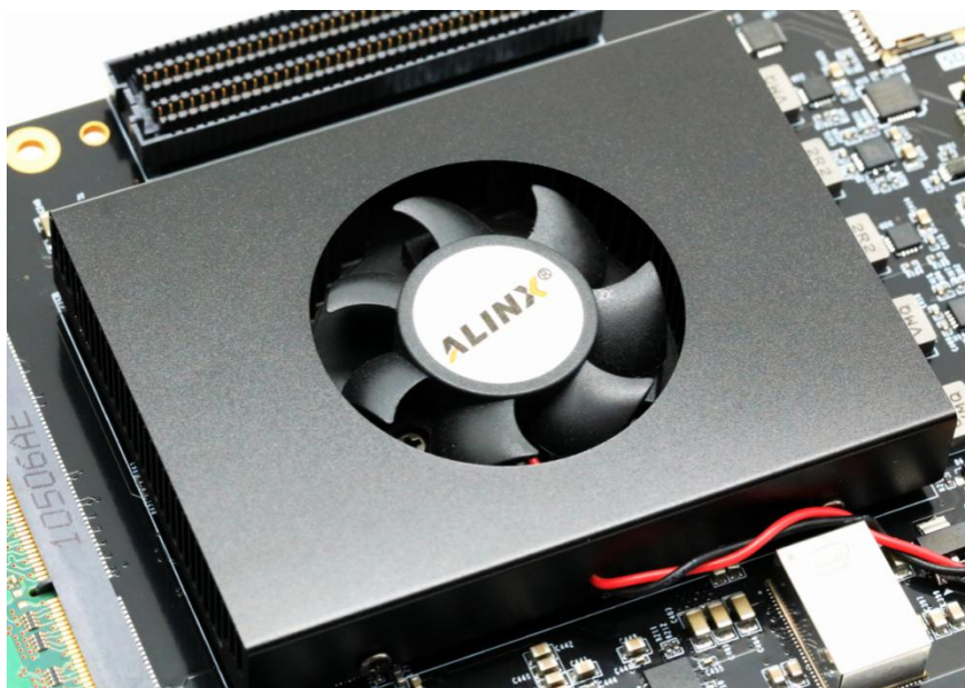
Figure 19-2: Fan on the FPGA Board
