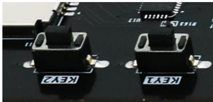
Figure 16-2: User Buttons on the FPGA Board
