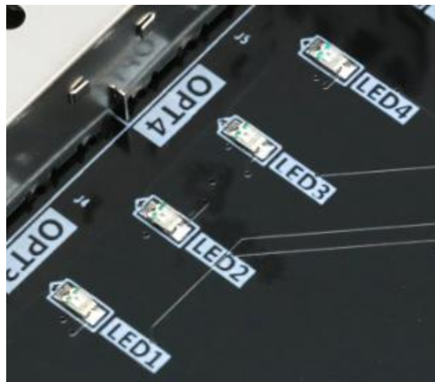
Figure 15-2: The User LEDs on the FPGA Board
