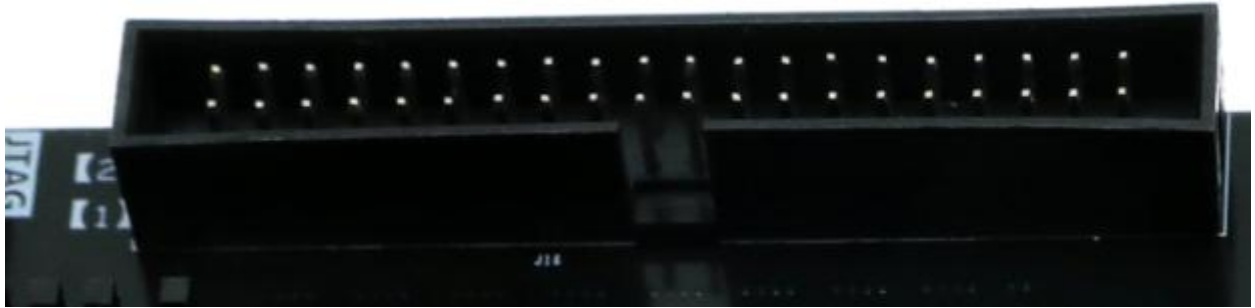
Figure 14-2: Expansion header J16 on the FPGA Board
