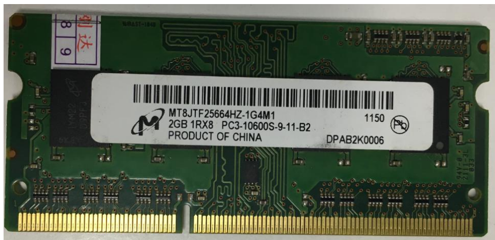
Figure 4-1: SODIMM memory test sample
